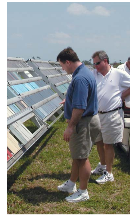
Covell inspects paint performance on metal panels at a test fence. He spends about one-third of his time on research and development.
