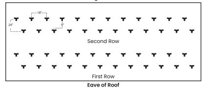
Example based on Everlast II® Roof Panels.
